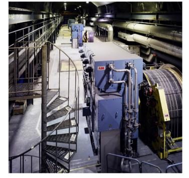
Certain ABB motors, whether variable speed drive (VSD) or direct online (DOL), boast rotors with heads weighing up to 130 tons and spanning four to eight meters in length. Enormous torque loads in cold conditions are brought to bear on the Ovako-sourced shafts throughout their speed range.
