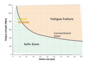
BQ-Steel and IQ-Steel have significantly smaller inclusions sizes compared to conventional steel. Note how the curve in the upperleft-hand corner is much steeper, meaning that the gain in fatigue strength is increasing exponentially.
