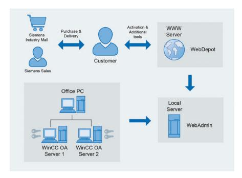
Customers can access all the information on their license options at any time. Locally, the CodeMeter Control Center service integrated in Simatic WinCC OA V3.17 provides users with an overview of all the licenses assigned to a device. Technical licenses and
